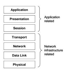
In a layered protocol architecture data flows vertically through the layers in each end station and horizontally over the network medium between end-stations. However, a peer to peer protocol is defined as the communication that takes place between two layers at the same level in different end-stations. Conceptually a peer to peer protocol operates horizontally and directly between the two layers as shown below.
