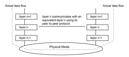
A peer to peer protocol does not consider data flow vertically within the model and simply assumes that the layer n protocol in one end-station communicates directly with the layer n protocol in a different protocol as if they were directly connected. This protocol is defined in terms of the commands and responses it issues together with a description of the protocol data unit format to be used.
