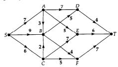
The shortest path algorithm is applied to the digraph D to find a shortest path from S to T.
