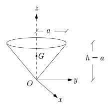
Given that the volume of the cone is  $\pi a^3/3$  show that the moment of inertia of the cone about about the x-axis, i.e.  $I_{Ox}$ , is  $3Ma^2/4$ .
