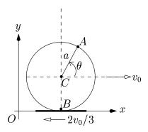
A is an arbitrary point on the circumference of the disc,  $\theta$  is the angle that the line AC makes with the horizontal, and B is the instantaneous point of contact between the disc and the conveyer belt, as shown in the diagram.
