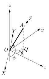
At time t,  $\phi$  is the angle between the negative z-axis and OA as shown, and  $\theta$  is the angle between the x-axis and OQ, where Q is the projection of A onto the xy-plane.
