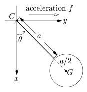
Using Routh's Rules and the Theorem of Parallel Axes, show that the moment of inertia of the pendulum about the axis Cz is  $19Ma^2/8$ . Verify your answer by direct integration, using the definition of the moment of inertia of a rigid body about the axis Cz.
