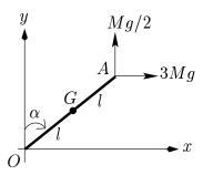
The centre of mass G of the rod is at a distance l from the origin O and the moment of inertia of the rod about the axis Oz is I. Assuming that the rod remains in the xy-plane at all times and that at time t it makes an angle  $\alpha$  with the vertical, show that:
