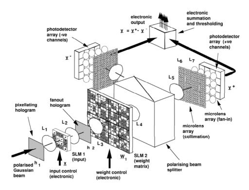
Explain how the optical system may be used to implement a Hopfield model of a neural network processor.
