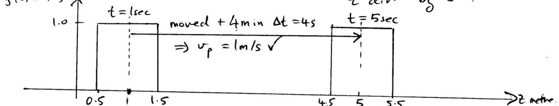
c) for  $t = 1 \text{ sec}$ ,  $v_p = -1 \text{ m/s}$ ,  $f(z - v_p t) = f(z + 1) = f(z)$  shifted in neg.  $z$  dir<sup>n</sup> by  $1 \text{ m}$ .
