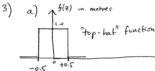
b) for  $t=1\text{sec}$ ,  $v_p=1\text{m/s}$ ,  $f(z - v_p t) = f(z - 1) = f(z)$  shifted in pos.  $z$  dir<sup>n</sup> by 1m.
