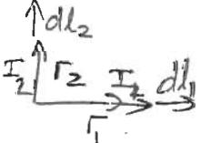
Force on  $dl_2$  is  $F_2 = \frac{\mu_0 I_1 I_2}{4\pi} \frac{dl_2 \wedge [dl_1 \wedge (r_2 - r_1)]}{|r_2 - r_1|^3}$
