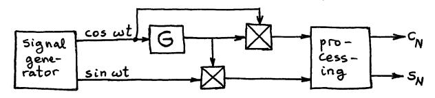
For several frequencies  $\omega$  in the relevant range, we compute in steady state, denoting  $T = \frac{2\pi}{\omega}$ ,  $C_N = \int_0^{NT} y(t) \cos \omega t \ dt = A_\omega \cdot \cos \phi_\omega \cdot \frac{NT}{2}$
