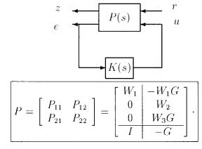
(c) Let the input to  $\Delta$  be  $\epsilon$  and the output from  $\Delta$  be  $\delta$ . Then  $\epsilon = -KS\delta$  and since KS is stable, the small gain theorem implies closed-loop stability if  $\|\Delta(j\omega)K(j\omega)S(j\omega)\| < 1, \forall \omega$ . Since K achieves the design specifications of Part (a),  $\|\Delta(j\omega)\| < |w_2(j\omega)|, \forall \omega$  is the maximal stability radius.
