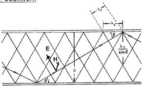
The above figure shows the side-view of a generic parallel-plate waveguide, supporting two plane-waves propagating between and reflecting off the wall plates. Propagation within the waveguide can only be maintained as long as  $\theta < \pi/2$ :
