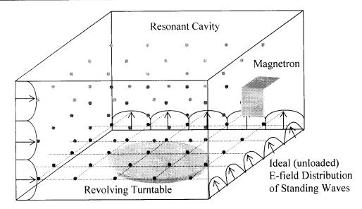
At 2.45 GHz the wavelength in free space is 122.5 mm. Therefore, there are approximately  $6 \times 6 \times 144$  points of E-field maxima (not shown above).
