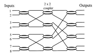
Somewhat surprisingly, the radiative star has far better performance than the coupler-based star, because variations in the accuracy of the power division of each coupler rapidly degrade the uniformity of the overall power distribution. These variations can arise from manufacturing, or changes in wavelength or polarisation. The radiative star is also simpler to lay out in mask-making.
