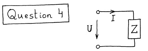
(a) If the circuit is a capacitor, then  $Z(s) = \frac{1}{Cs}$ , which is proper but not slable. If the circuit is an inductor, then Z(s) = Ls, which is not proper, hence not a stable transfer function. If Z would have poles in  $C_+$ , then the voltage produced by an initial state (with I=0) would grow without bound. This is impossible, since there are no sources in the circuit.
