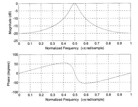
The filter is bandpass with a centre frequency of pi/2. The magnitude of frequency response will exhibit this behaviour if poles are located on the imaginary axis, relatively close to, but inside, the unit circle.
