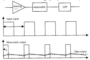
The reading is the DC component of the output, namely:
