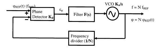
Used at lower frequencies and when ease of adjusting the multiplication factor is desired.
