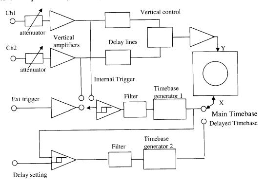
The horizontal sweep system of the oscilloscope consists of the trigger, a one shot sawtooth generator called the **timebase generator** which is of sufficient amplitude for the beam to span horizontally the screen. A horizontal magnification feature, often provided, simply adds a post amplifier to the timebase generator.
