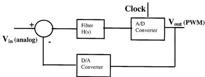
With H(s) 1<sup>st</sup> order LPF at 50 kHz. Then the resolution gain is 1.5bit/bit of oversampling, i.e. only need 5 bits of oversampling (3.2 MHz) to obtain 10 bit resolution.
