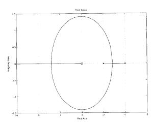
roots of  $\frac{dG(s)}{ds} = 0$  and are equal to  $\boxed{-3 \pm \sqrt{2} \sim -4.4, -1.6}$ . The asymptote is at  $180^{\circ}$ .
