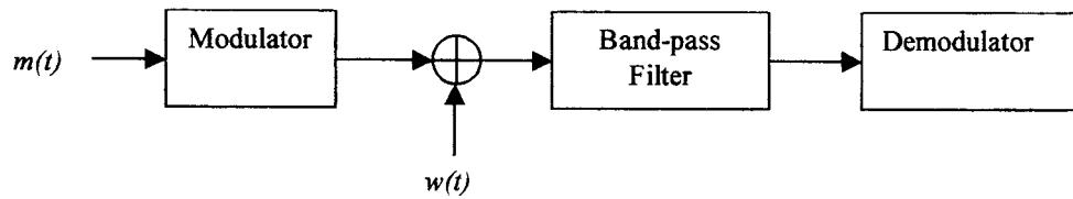
where  $m(t)$  is the base-band message signal,  $w(t)$  is additive zero-mean Gaussian noise with a flat power spectral density of height  $N_o / 2$ , and the band-pass filter has a pass band (of appropriate width) centered on the carrier frequency  $\omega_c$ .
