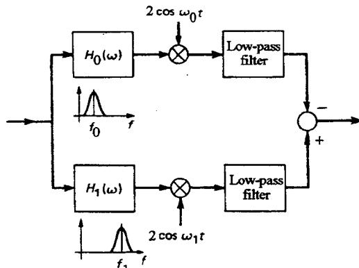
Also consider the synchronous PSK detector shown in the figure below, where the input to the detector is a PSK signal.
