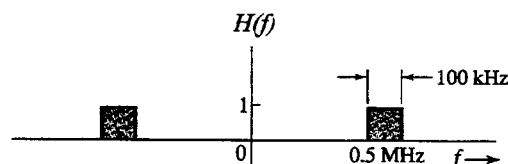
Draw the power spectral densities of the base-band components  $n_c(t)$  and  $n_s(t)$  at the output of the filter. Also calculate the average power in each base-band component.
