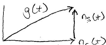
where we see that  $n_c(t)$  is in-phase ~~with~~ component of rotating phasor &  $n_s(t)$  is  $90^\circ$  out of phase (in quadrature) with rotating phasor.
