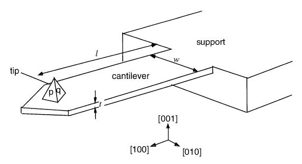
(b) The tip is fabricated a distance l from the cantilever support. The cantilever has width w and thickness t. Show that the relevant second moment of inertia, I, for calculating the deflection of the cantilever is given by
