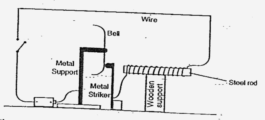
(a) Explain why the metal striker is pulled towards the steel rod when the switch is closed.
