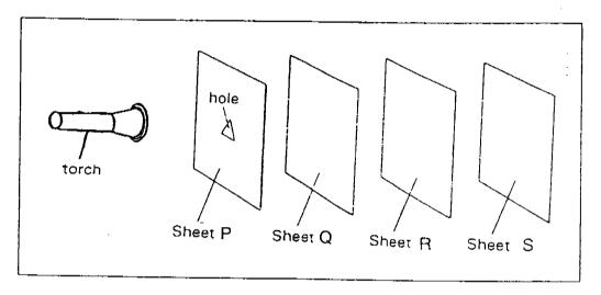
Sheets P, Q, R and S were arranged in a straight line. When the torch was switched on, a bright triangular patch of light was seen on Sheet R only.
