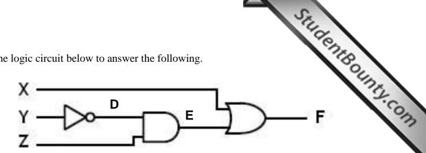
Complete the **truth table** for the above logic circuit. a.
