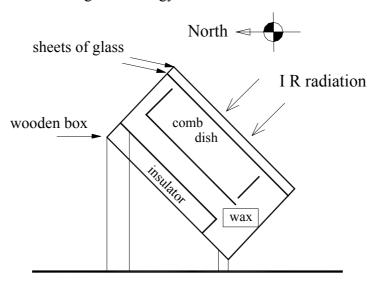
The above diagram shows how beekeepers in Malta use the Sun's IR rays to extract pure beeswax from old empty honeycombs. The box is called: A Solar Wax Extractor.
