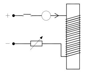
The diagram shows an electromagnet. It is used to pick up iron staples.
