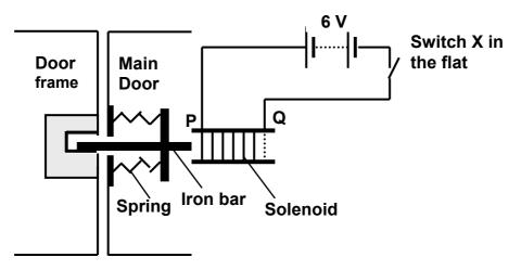
When switch X in the flat is closed, the iron bar moves towards end P of the solenoid and out of the door frame, allowing the main door to be opened.
