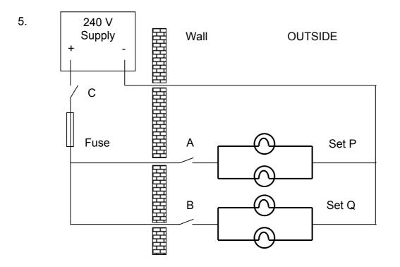
An outdoor lighting device consists of two sets of identical lamps. Each set containing 2 lamps in parallel. Each lamp is rated 240V, 60W.
