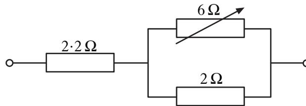
(i) Calculate the resistance of the **parallel** branch shown above.
