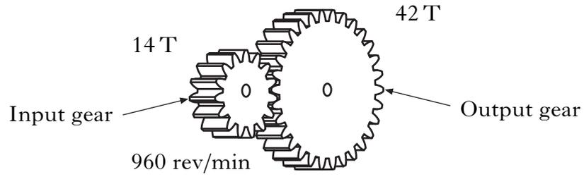
(c) Calculate the speed of the output gear when the input gear rotates at 960 rev/min.
