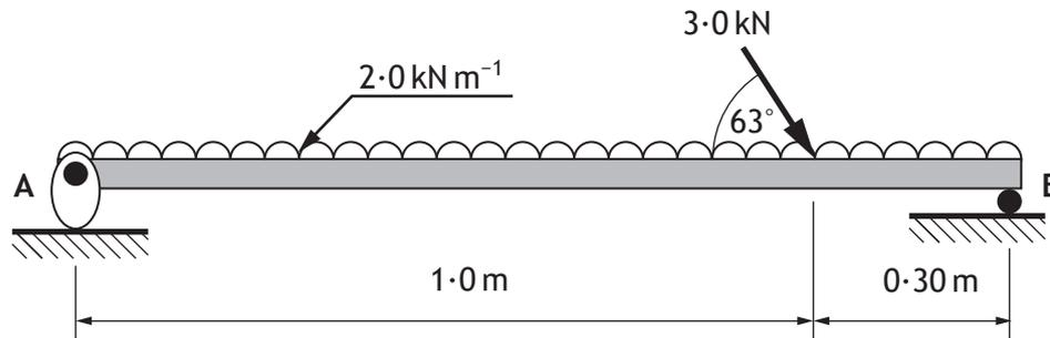
(d) Determine the magnitude and direction of the reaction at A.
