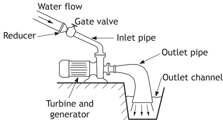
The engineer measured the electrical output from the generator to be 22 A at 230 V. The mass of water flowing through the inlet pipe into the generator was 2500 kg every second at an average flow rate of  $3.2 \text{ ms}^{-1}$ .
