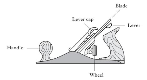
Describe how the plane can be adjusted to:
