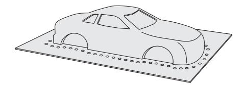
Sloping sides, rounded corners and small holes are all features of the pattern.
