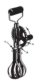
In the figure above, a simple gear arrangement is shown. If there are 32 teeth on the large vertical wheel A, 8 teeth on horizontal wheel B, and 8 teeth on horizontal wheel C, one complete revolution of wheel A results in
