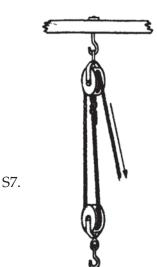
In the figure shown above, the pulley system consists of a fixed block and a movable block. The theoretical mechanical advantage is
