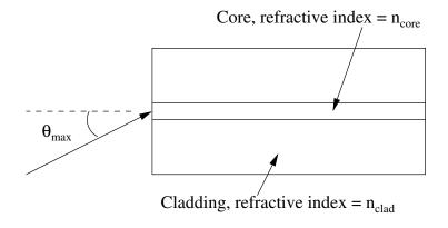
Light may only be transmitted along the fibre if the incident angle of the light is less than a maximum angle  $\theta_{max}$ . By using your expression from part (b) and Snell's Law, or otherwise, derive an expression for  $\theta_{max}$  in terms of the core and cladding refractive indices only.
