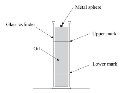
(a) The diagram shows a glass cylinder containing oil. A student holds a metal sphere at the surface of the oil and then releases it. The sphere accelerates at the start and then reaches a constant speed before reaching the upper mark on the cylinder. It then continues at this speed until it reaches the bottom of the cylinder.
