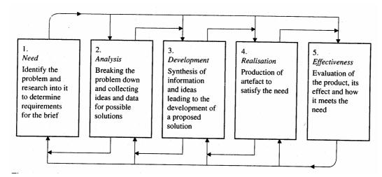
The arrows show that it is not always a linear series, that there is frequent looping back, particularly, an ongoing reappraisal of the nature of the need. The arrows at the top showing forward links indicate for example that when considering the nature of the need (box 1) the resources available for realisation (box 4) and the constraints must be kept in mind. Similarly, the likely effects (box 5) need to be anticipated at every stage.
