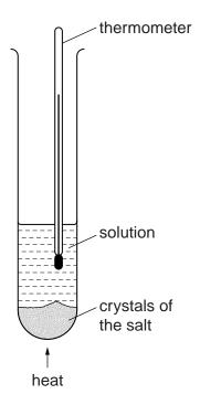
10 g of water is placed in a boiling tube and 7.0 g of ammonium chloride is added.
