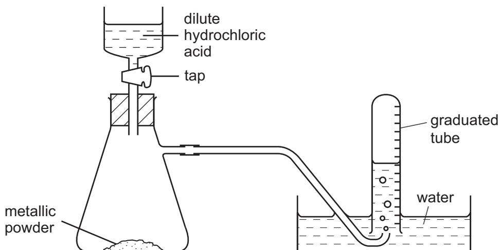
The experiment is carried out three times, using the same mass of powder each time but with different powders:
