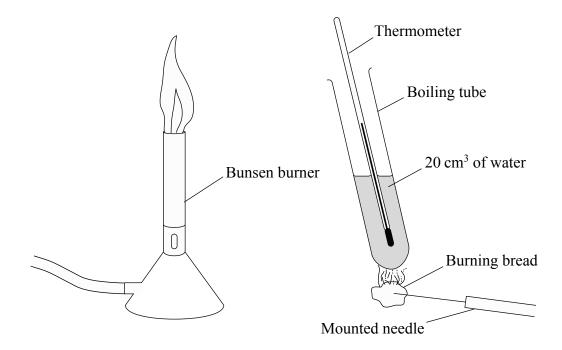
The temperature of the water in the boiling tube at the start was  $15\,^{\circ}\text{C}$  and the mass of the bread was  $0.4\,\text{g}$ . Bethany placed the bread on the mounted needle, lit the bread in the Bunsen flame then moved it as quickly as possible and held it under the boiling tube. After the bread had completely burned, the temperature of the water was  $38\,^{\circ}\text{C}$ .
