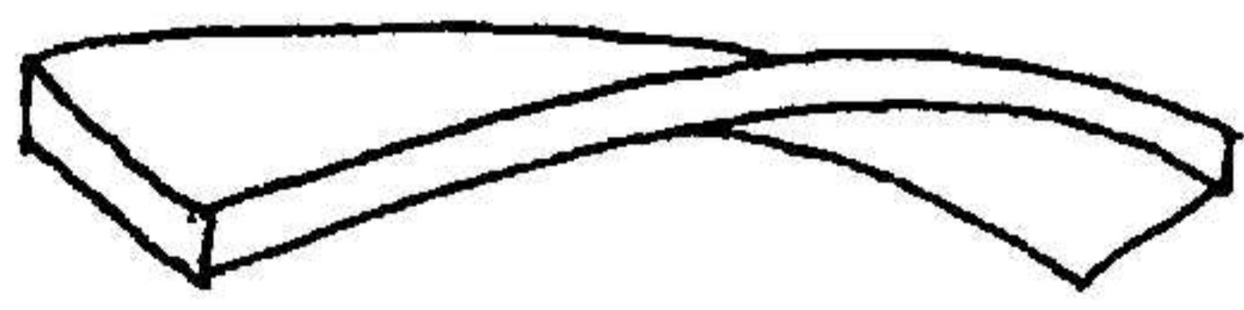
A simple line drawing of a rectangular board that is curved upwards along its length, representing a bowed or warped piece of wood. | (1)         |
