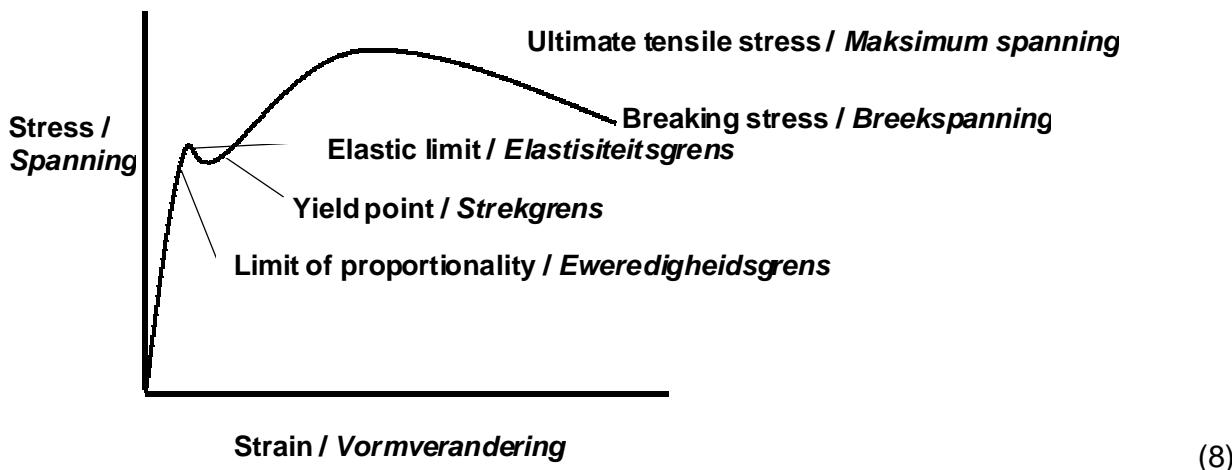
$$3.4 \quad (a) \quad \begin{aligned} \text{Strain} &= \frac{\text{Change in length/veranderin g in lengte}}{\text{Original length/Oorspronklike lengte}} \\ \text{Vormverandering} &= \frac{0,124}{2\ 000} \end{aligned}$$
