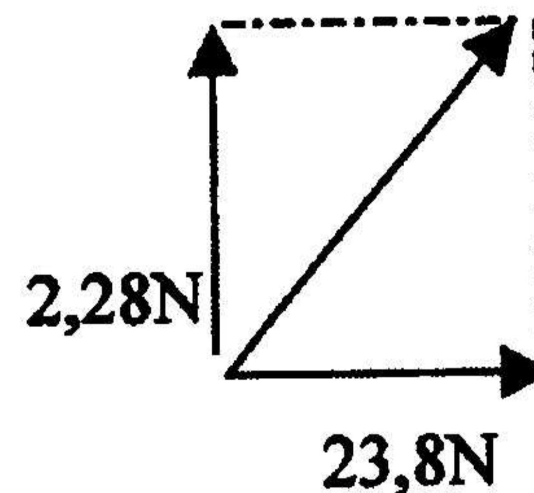
$$\begin{aligned} \tan \vartheta &= \frac{2,28}{23,39} \\ &= 0,0957 \\ \vartheta &= 5,47^\circ \end{aligned}$$
