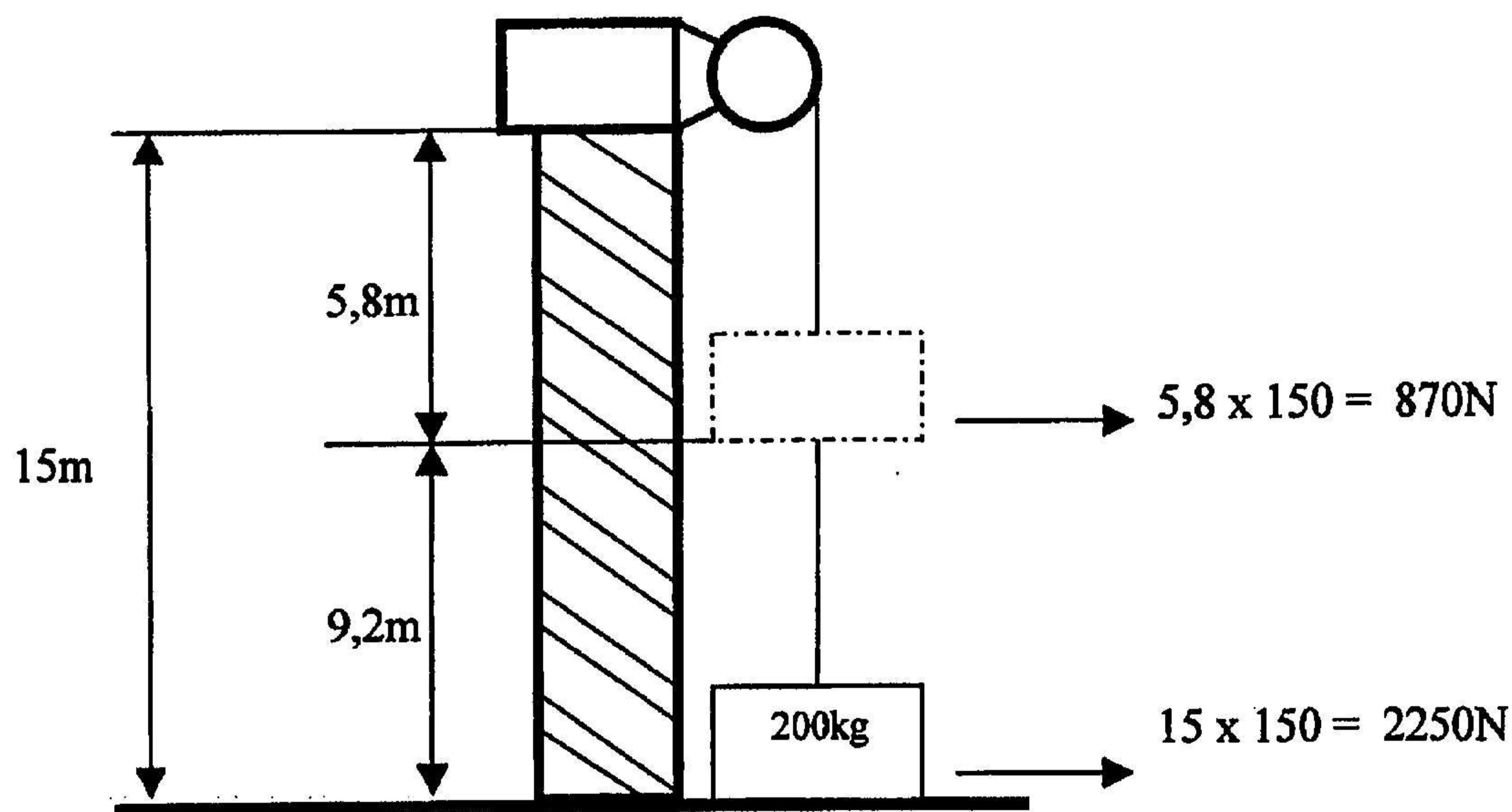
$$\begin{aligned}\text{Work done (W)} &= F \text{ for lift} + \text{average } F \text{ for cable} \times \text{distance} \\ &= 2000 \text{ N} + \frac{2250 + 870}{2} \times 9,2 \\ &= \underline{\underline{32\ 752 \text{ J}}}\end{aligned} \quad (8)$$
