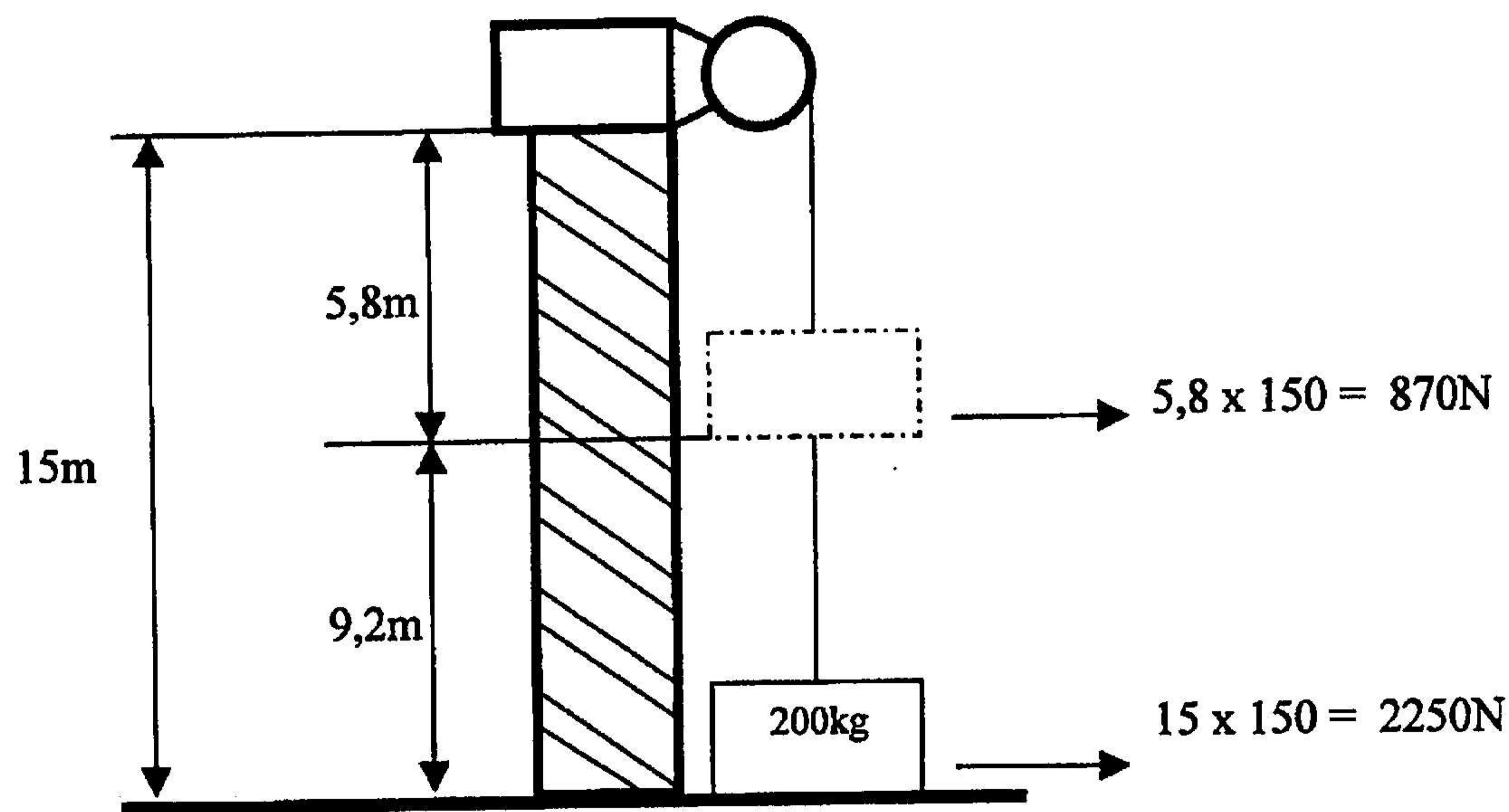
$$\begin{aligned}\text{Arbeid verrig (W)} &= F \text{ vir hysbak} + \text{gem } F \text{ vir kabel} \times \text{afstand} \\ &= 2\ 000 \text{ N} + \frac{2250 + 870}{2} \times 9,2 \\ &= \underline{\underline{32\ 752 \text{ J}}}\end{aligned}$$
