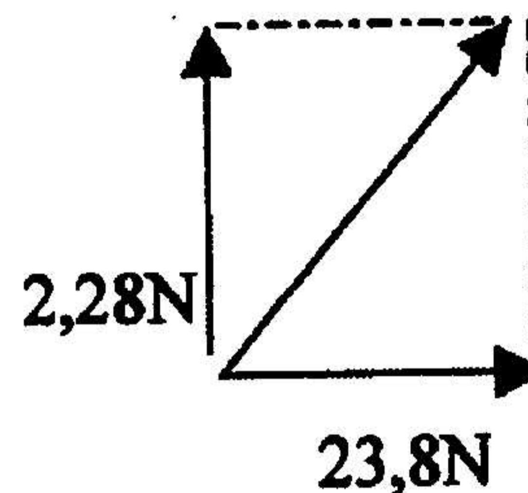
$$\begin{aligned} \tan \Theta &= \frac{2,28}{23,39} \\ &= 0,0957 \\ \Theta &= 5,47^\circ \end{aligned}$$
