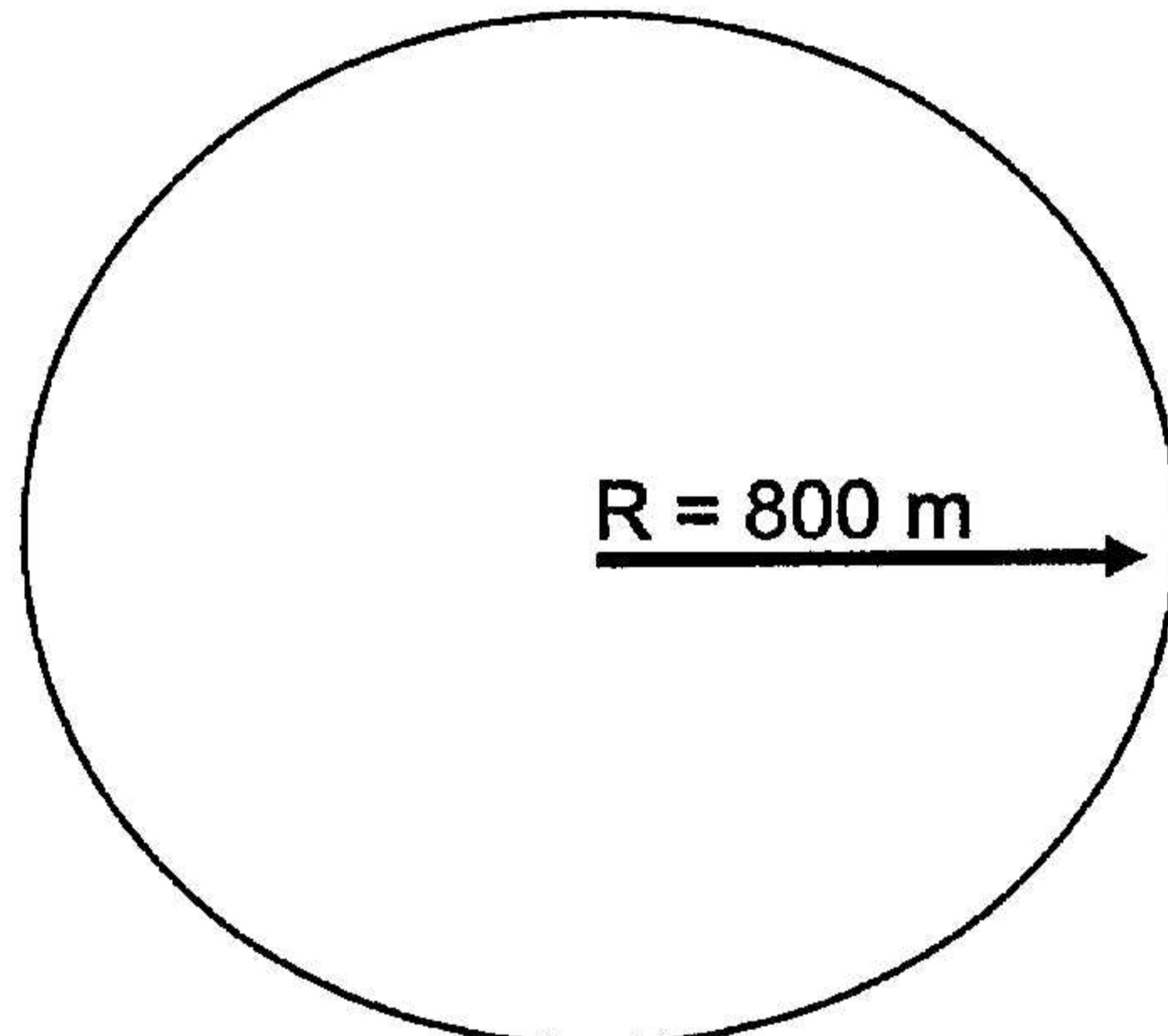
$$\begin{aligned} 56 \text{ km/h Omtrek van sirkel} &= 2\pi r \\ &= 2 \times \pi \times 800 \\ &= 5026,5 \text{ m} \end{aligned}$$
