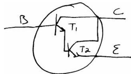
Biasing arrangement: Positive on base, Positive on Collector and Negative on Emitter
