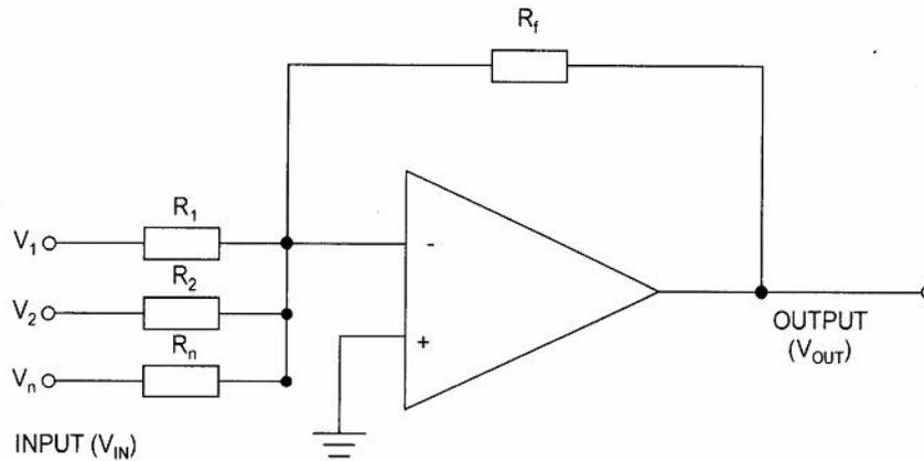
$$V_0 = \left( \frac{V_1 R_f}{R_1} + \frac{V_2 R_f}{R_2} + \dots \right)$$
