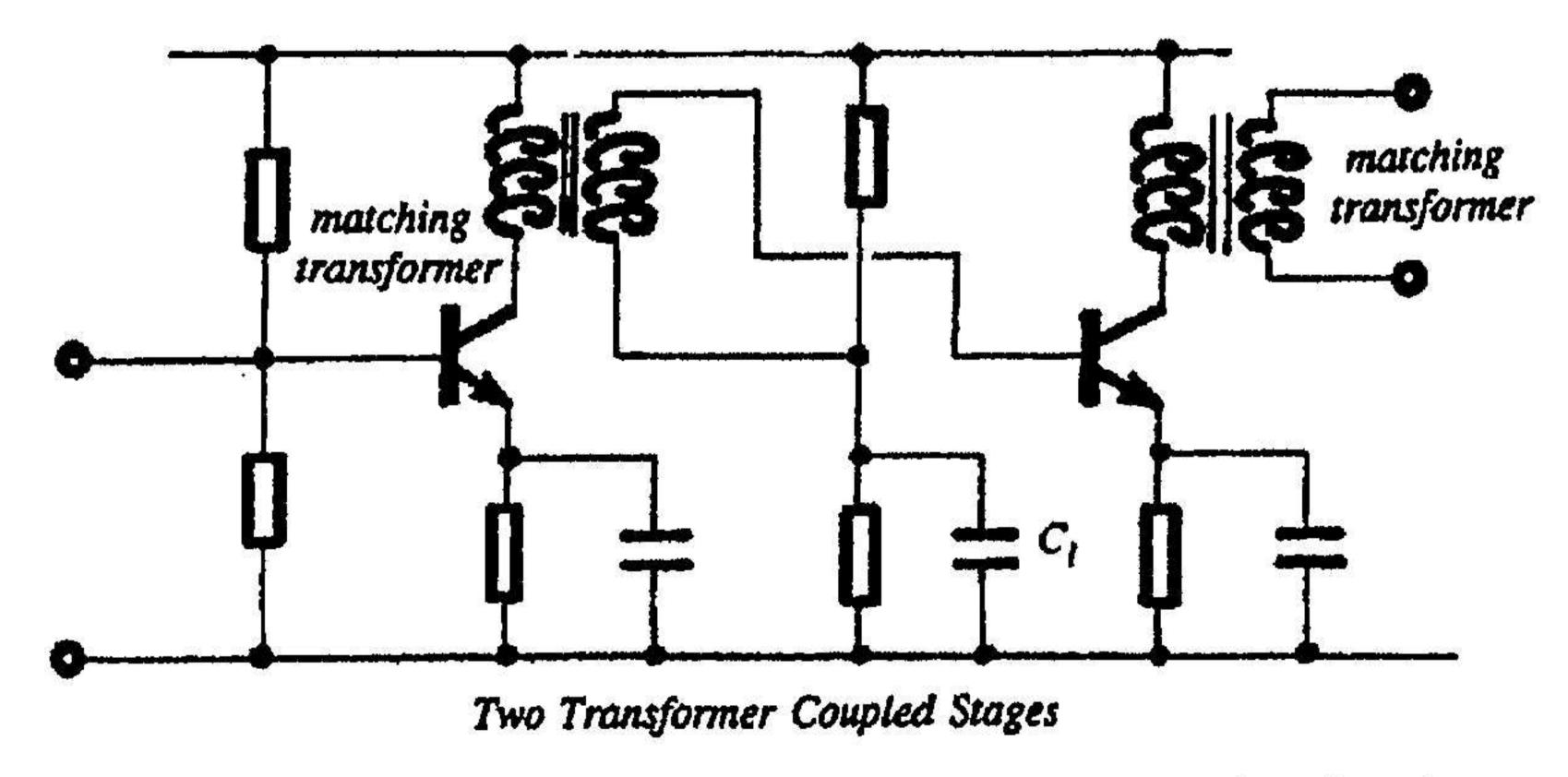
A transformer coupled circuit is expensive to build, large in size but easy to design. It is often used in circuits requiring large current outputs or where two phase-split outputs are required as in a push-pull amplifier (see later). It is more efficient than RC coupling as the primary coil's resistance (which replaces the collector resistance) has a much lower value and therefore causes less do power loss for the stage.
