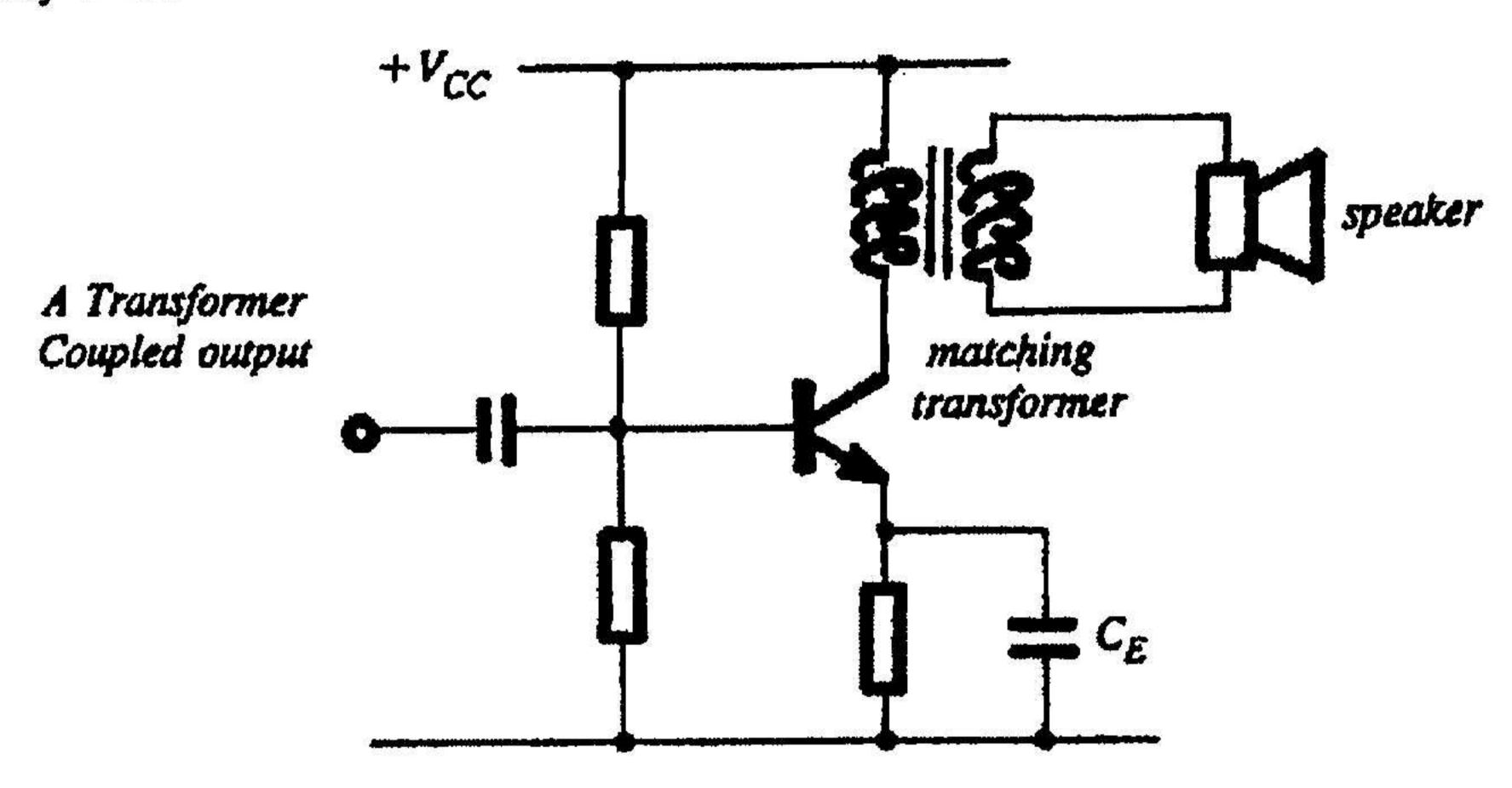
Because they are made from coils of copper wire, the resistance of transformer windings is very low. When used as the collector load in a transistor amplifier this creates a very steep (almost vertical) load line on the output characteristic, which creates very-high-current currents with a small voltage output. This is useful for driving low-impedance loads such as relays, loudspeakers and motors.
