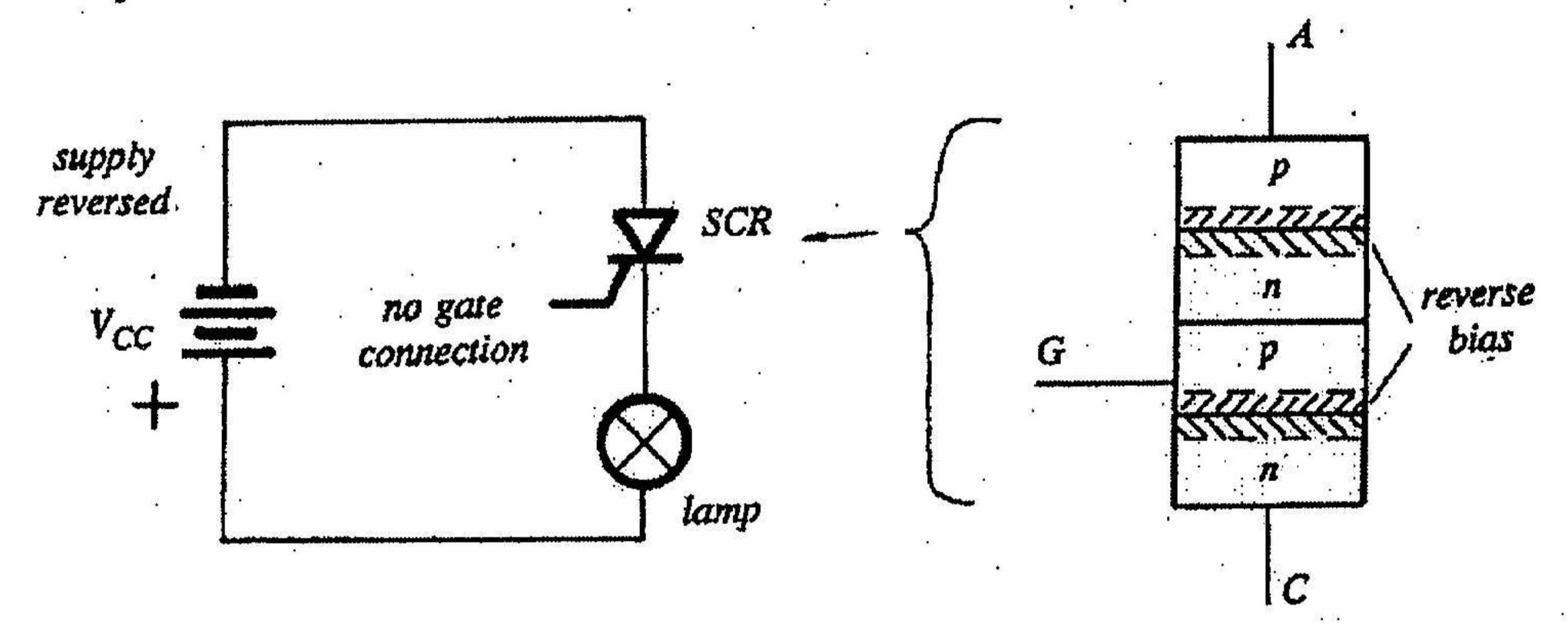
For conduction to occur the anode-cathode must first be forward biased just like a normal diode. Then a trigger signal is applied to the gate. This trigger voltage must be large enough to break down the middle reverse bias junction. Once all three junctions are forward biased anode current will flow through the SCR and energise the load.
