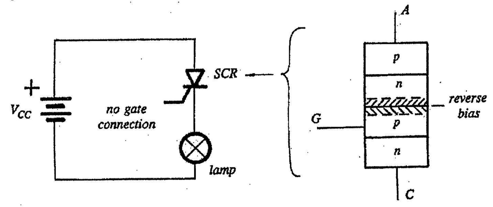
2. In the reverse direction with the anode negative and the cathode positive, the two outer parjunctions are reverse biased and the centre junction is now forward biased. No conduction.
