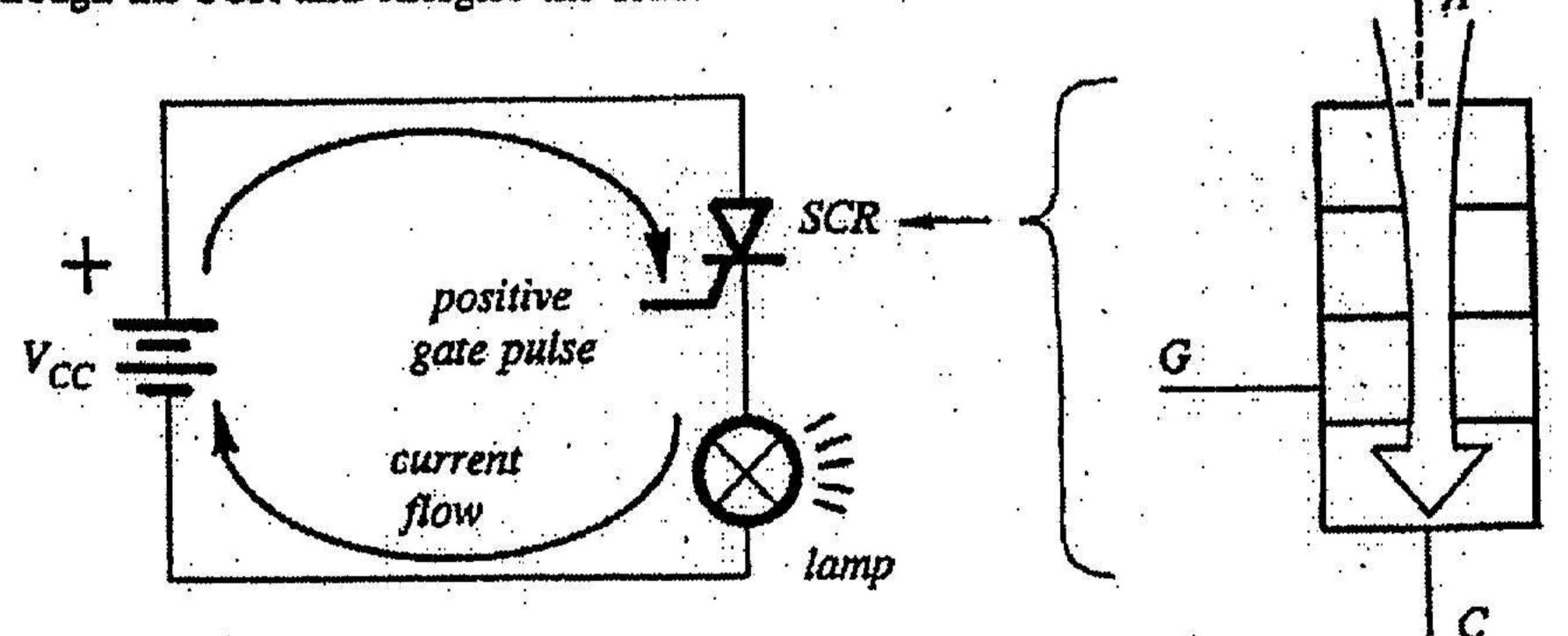
Once the SCR goes into conduction the gate is no longer needed and it looses all further control over the SCRs operation.
