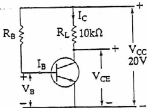
$R_B$  provides the voltage to bias the EB of the transistor. The input coupling capacitor blocks DC and allows AC to pass through. A constant DC flows through  $R_L$ . This constant current develops a constant voltage across the output of the transistor. A positive pulse on the base increases the forward bias conditions and turns the transistor harder on allowing more current to flow and increase the output wave 180 degrees out of phase with the input wave.
