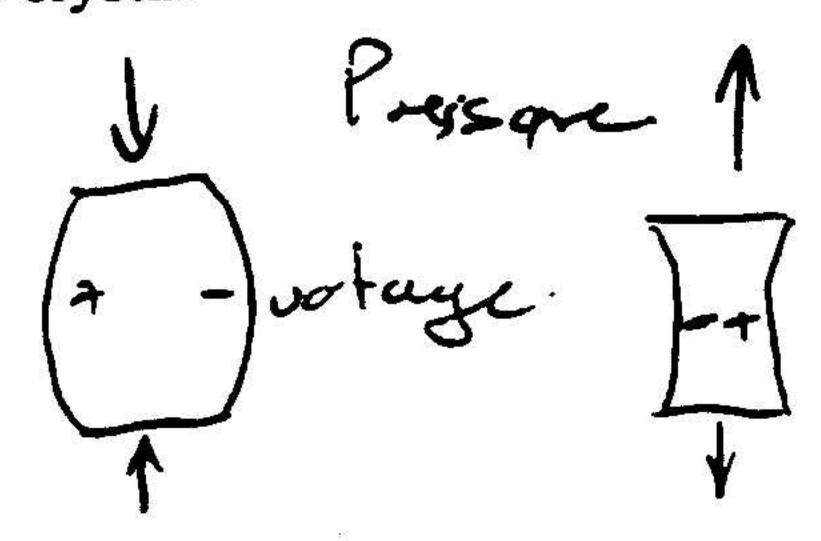
9.3 To stabilize the frequency of the oscillator. It acts as a filter for harmonic frequencies.
