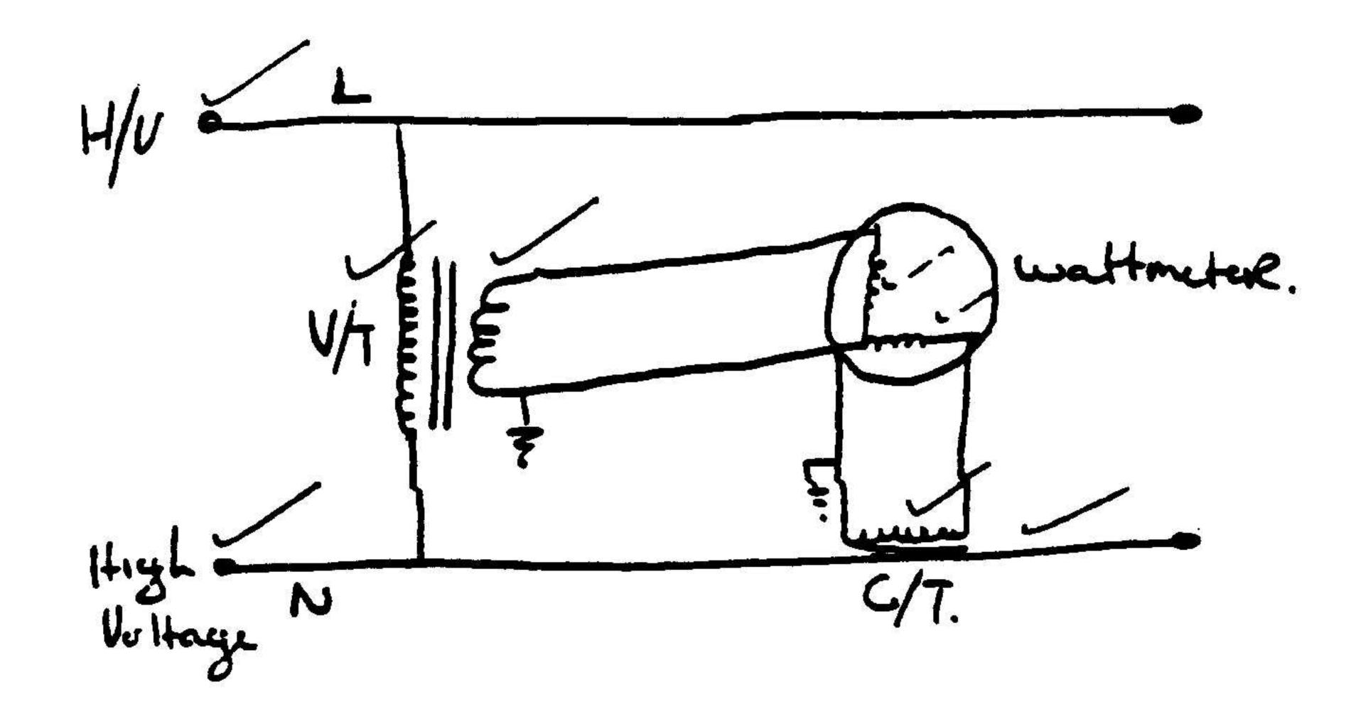
3.3 A transformer operates on the principle of Faraclay's kW. If no change in voltage OR current takes place, no induction can occur therefore a transformer operates on A/C.
