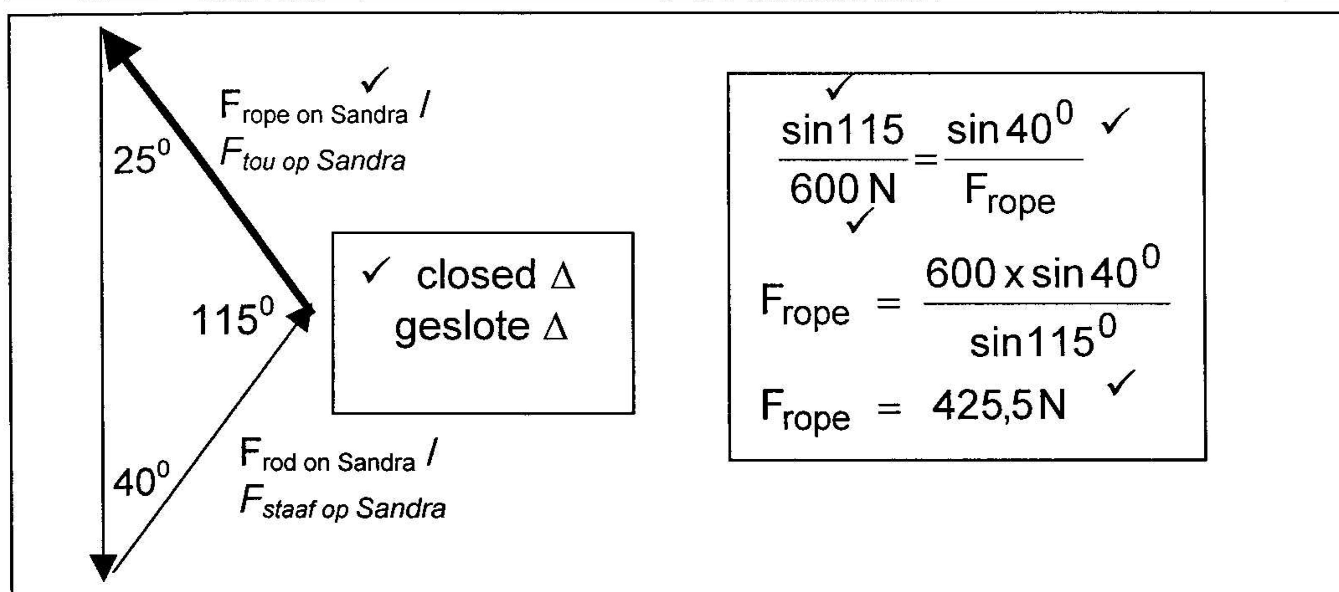
**BY CONSTRUCTION / BY SKAALTEKENING**orientation ✓
