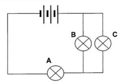
Which ONE of the following combinations correctly represents the brightness of bulbs A and B, compared to their original brightness, if bulb C is removed?
