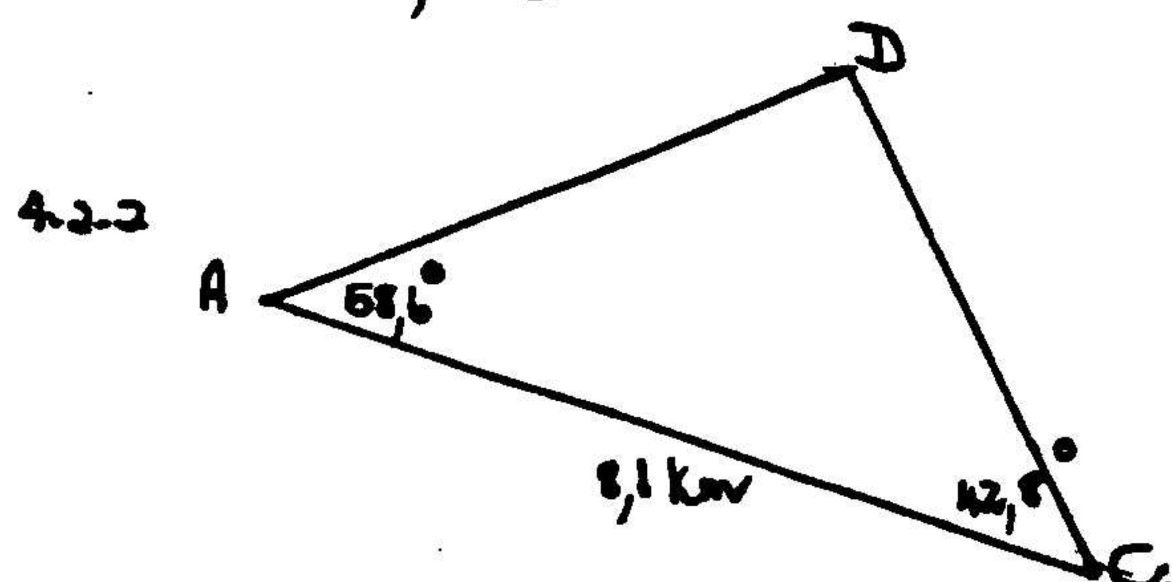
$$\begin{aligned} D &= 180^\circ - (58,6^\circ + 42,8^\circ) \\ &= 180^\circ - 101,4^\circ \\ &= 78,6^\circ \quad (1) \end{aligned}$$
