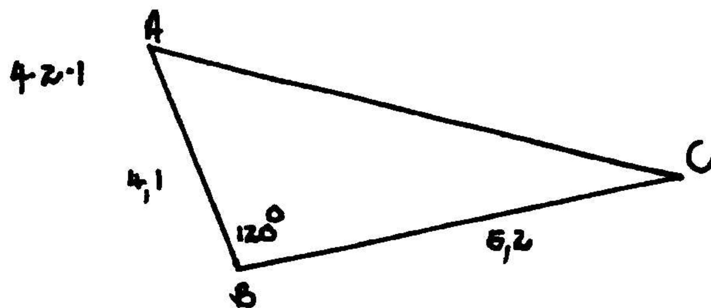
$$\begin{aligned} AC^2 &= AB^2 + BC^2 - 2(AB)(BC) \cos B \quad (1) \\ &= (4,1)^2 + (5,2)^2 - 2(4,1)(5,2) \cos 120^\circ \quad (1) \\ &= 16,81 + 25,92 - 42,64(-0,5) \quad (1) \\ &= 43,85 + 21,32 \\ &= 65,17 \quad (1) \end{aligned}$$
