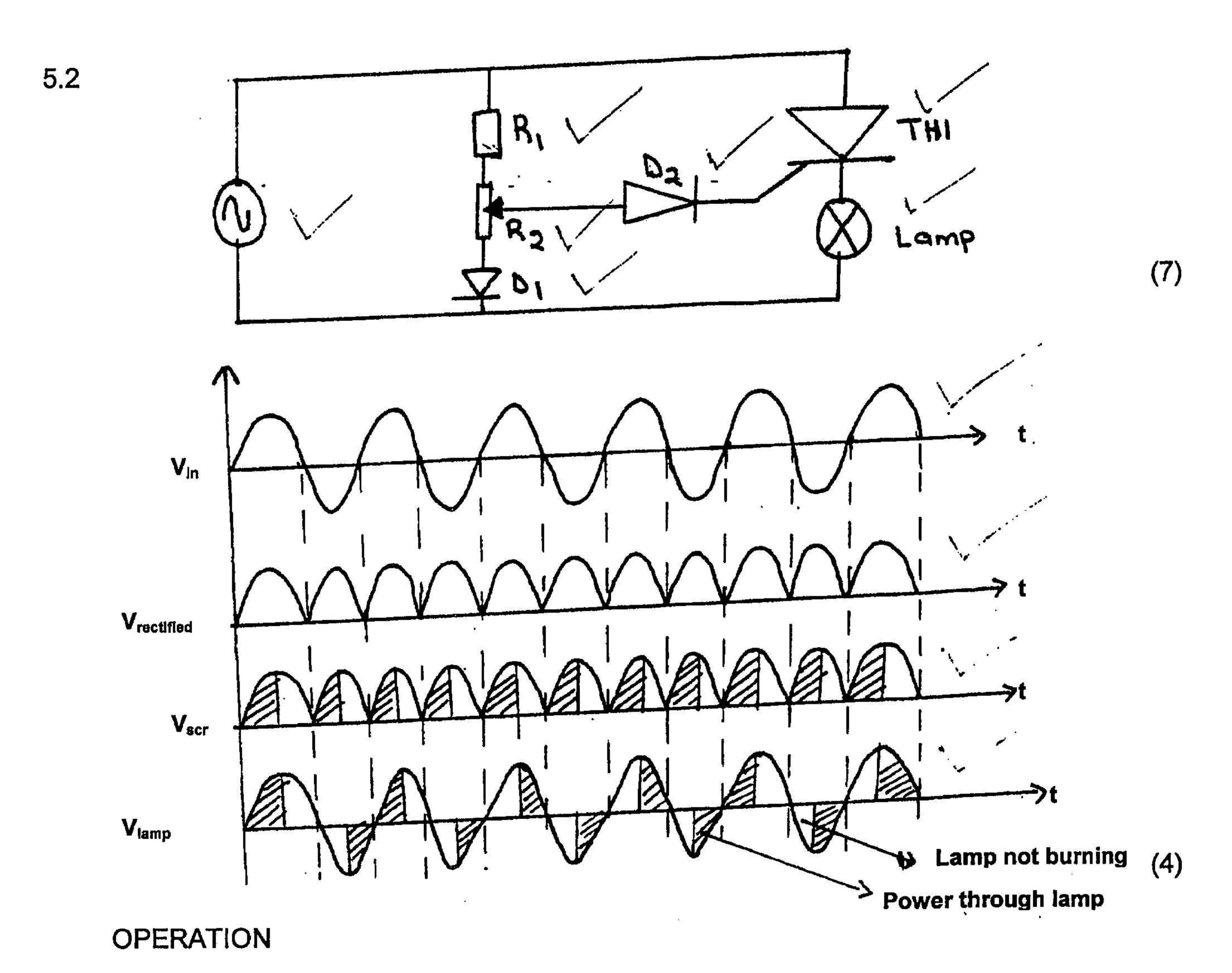
The. trigger angle is controlled by resistor R₂√
