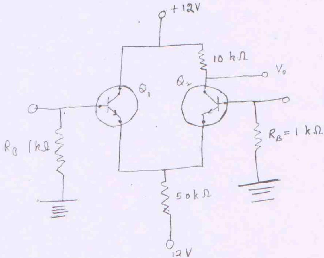
Assuming that  $Q_1$  and  $Q_2$  have identical  $\beta_{dc} = 100$ , find the emitter currents  $I_B$  and input bias currents  $I_E$  in each of the transistors. Using the Ebers-Moll equation  $I_c(V_{BE})$ , find the differential gain and common mode gain of the above amplifier.
