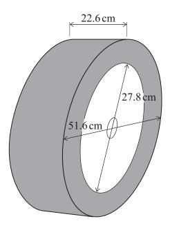
The diagram shows a racing car wheel with a tyre around it.
