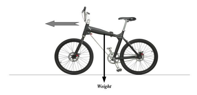
A bicycle is free wheeling along a flat road in the direction shown. The bicycle has a weight of 350N.
