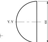
3. Draw the profile shown below, using geometrical methods to determine the centres of the arcs.
