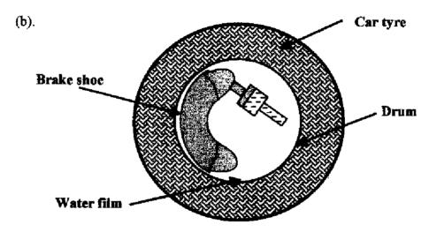
The diagram shows a part of the braking system in a motor car. The brake shoe and drum get soaked in rainwater as the car passes through a flooded area. The work done by friction as the brake pad is pressed against the drum is changed to heat energy.
