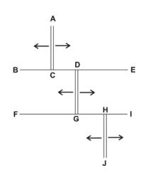
The above figure is a plan view showing a segment of the boundary zone between two plates. The arrows represent the velocity of movement across parts of the boundary. BE and FI are fault scarps that apparently displace the segments AC, DG and HJ.
